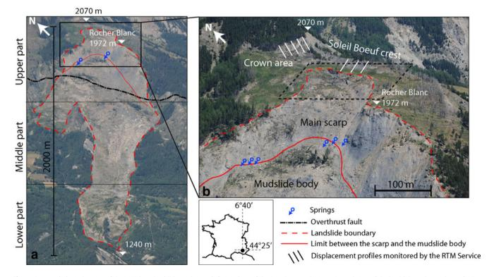
**Fig. 1** Geomorphological setting of the La Valette landslide on the south-facing slope of the Barcelonnette basin. **a** General view of the landslide to the northeast. **b** View of the main scarp and the crown areas; the dashed line delineates the area investigated by TLS and seismic tomographies. The displacement profiles measured by the "Restauration des Terrains de Montagne, RTM" office to monitor the retrogression of the crown are also indicated
