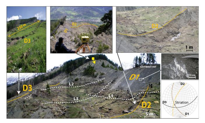
Fig. 5 Photographs of the crown area presenting three major discontinuities D1, D2, and D3 and the associated stereonet (equal angle, lower hemisphere). Striations are observed on D1. The location of the TLS (*yellow square*) and the seismic profiles (L1, L2, and L3) are also indicated
